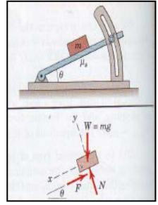
Dividing the first equation by the second gives  $F/N = \tan \theta$ . Since the maximum angle occurs when  $F = F_{\text{max}} = \mu_s N$ , for impending motion we have
