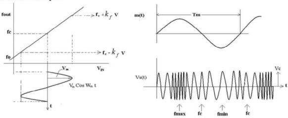
The output frequency varies 'gradually' from  $f_c$  to  $(f_c + k_f V_m)$ , through  $f_c$  to  $(f_c - k_f V_m)$  etc.
