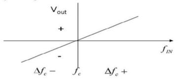
The important point is that  $V_{OUT} = K k_f V_{IN}$ . If  $V_{IN} = m(t)$  then the output contains the message signal m(t), and the FM signal has been demodulated.
