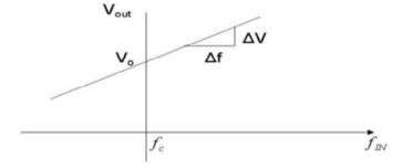
We define  $V_o$  as the output when  $f_{IN} = f_c$ , the nominal input frequency.
