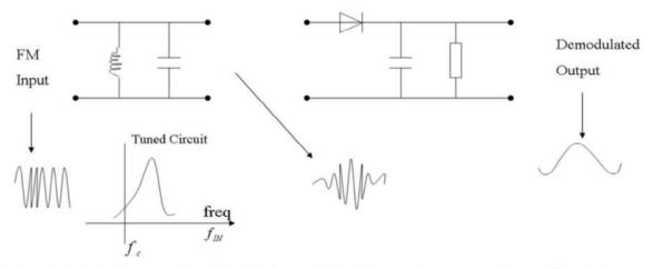
• The tuned circuit is tuned so the f<sub>c</sub>, the nominal input frequency, is on the slope, not at the centre of the tuned circuits. As the FM signal deviates about f<sub>c</sub> on the tuned circuit slope, the amplitude of the output varies in proportion to the deviation from f<sub>c</sub>. Thus the FM signal is effectively converted to AM. This is then envelope detected by the diode etc to recover the message signal.
