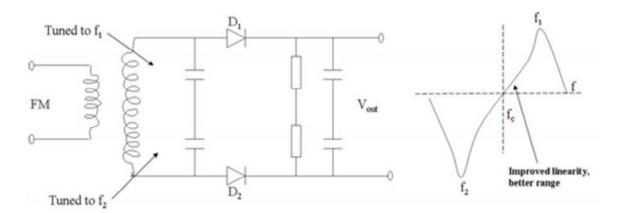
This gives the composite characteristics shown. Diode  $D_2$  effectively inverts the  $f_2$  tuned circuit response. This gives the characteristic 'S' type detector.
