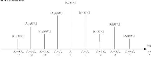
The amplitudes drawn are completely arbitrary, since we have not found any value for  $J_n(\beta)$  – this sketch is only to illustrate the spectrum.
