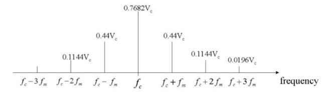
Bandwidth of Significant Spectrum =  $6 f_m$
